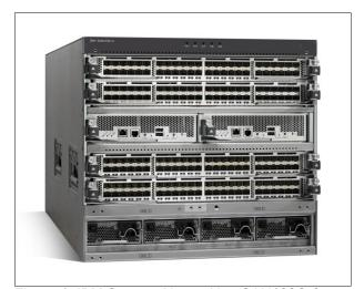
Figure 1. IBM Storage Networking SAN192C-6
